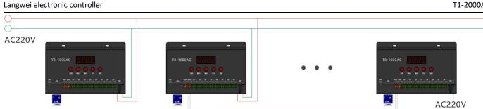
During hybrid synchronization, all controllers using high-voltage synchronization comply with the requirements of high-voltage synchronization, and they are all hosts; All controllers using cascade synchronization meet the requirements of cascade synchronization, and they are slaves.
